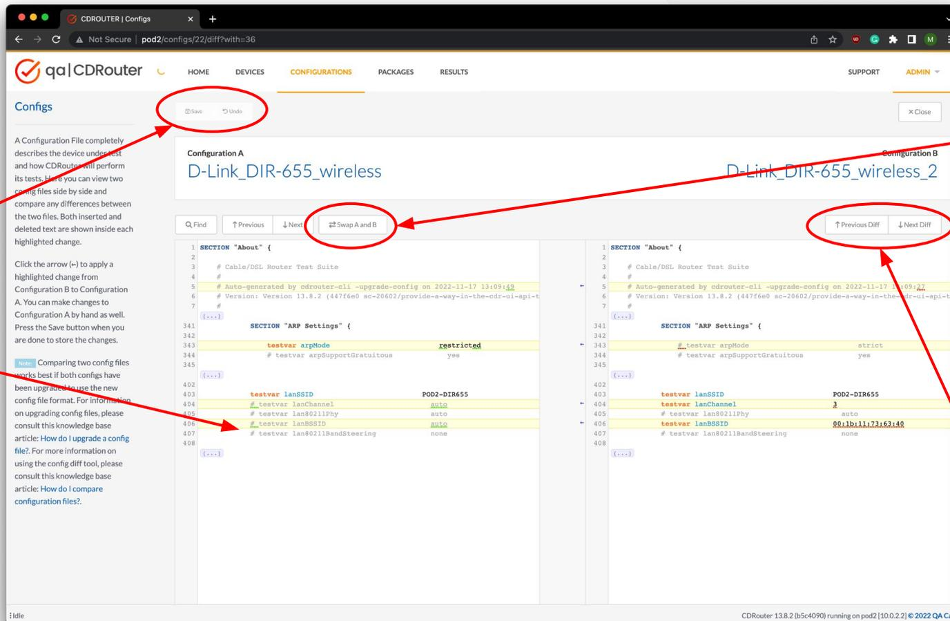
Configuration A and B may be swapped, making it possible to edit either configuration from the diff view.
