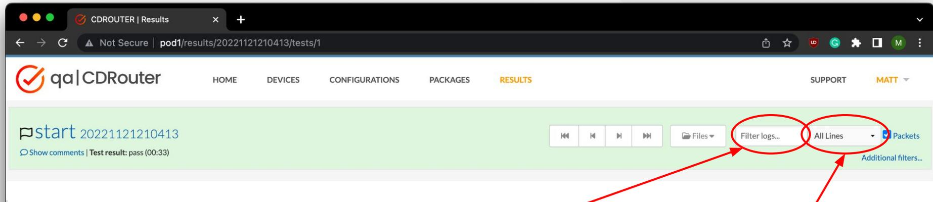
This text box allows filtering of the log file using keywords.
